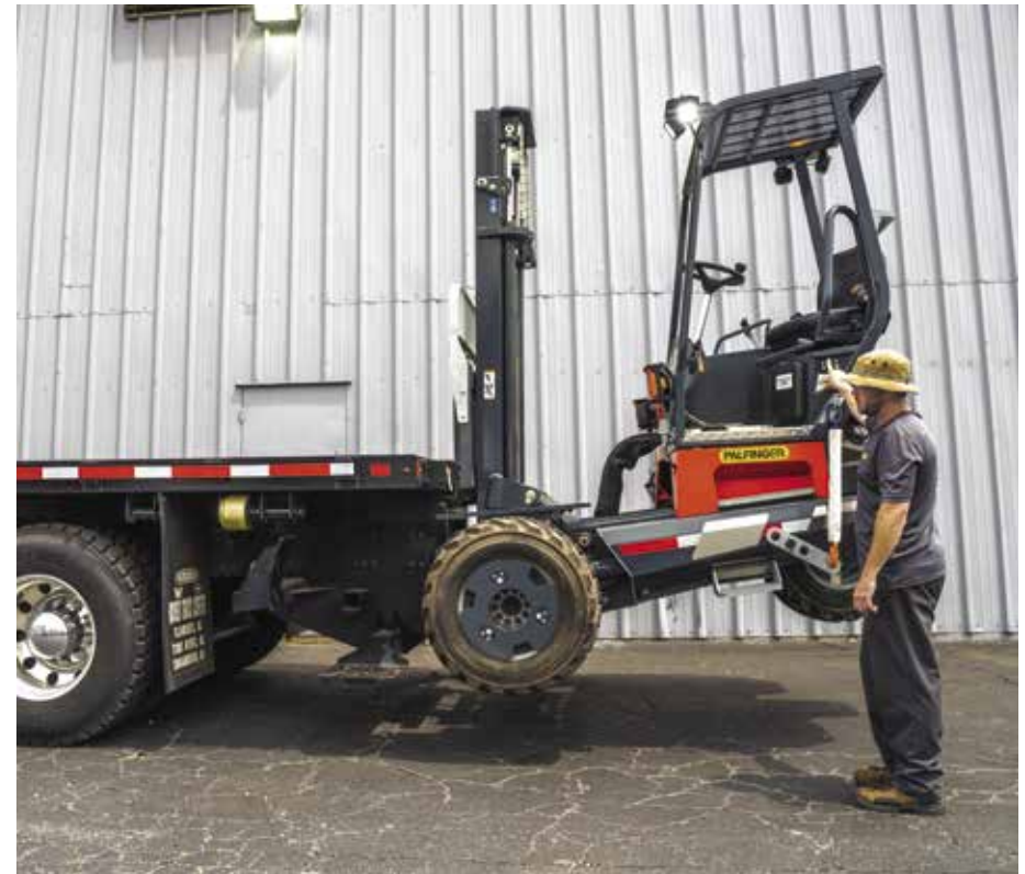
Lower the forklift and go...use the three switches to TILT, EXTEND and LOWER the machine to the ground
